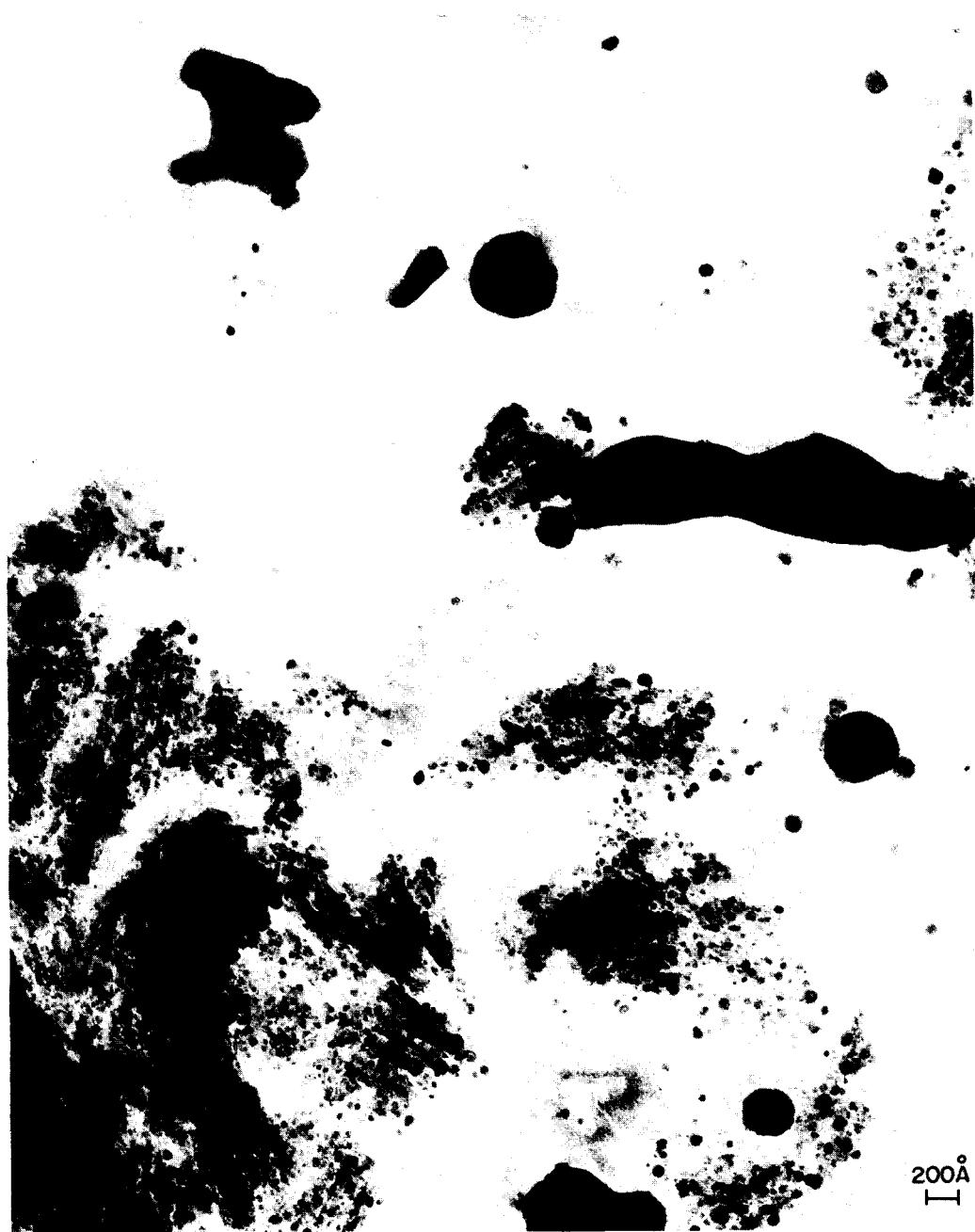
FIG. 4C. Extraction replication showing mixture of catalyst particles from 10 Å to 1 \mu\text{m} in size.
