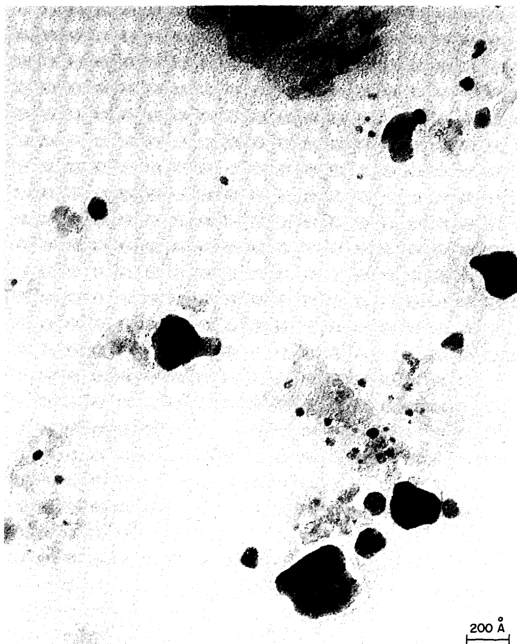
FIG. 5B. Catalyst particles after beam heating (coalesced).
