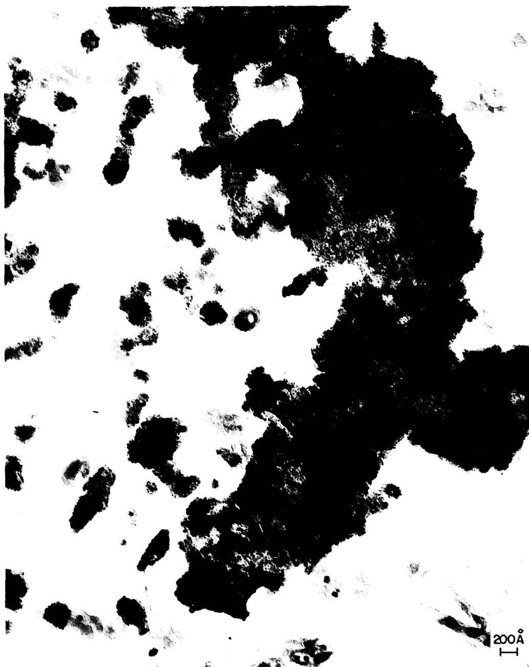
FIG. 4A. Sample prepared by extraction replication showing isolated clusters and massive aggregates.
