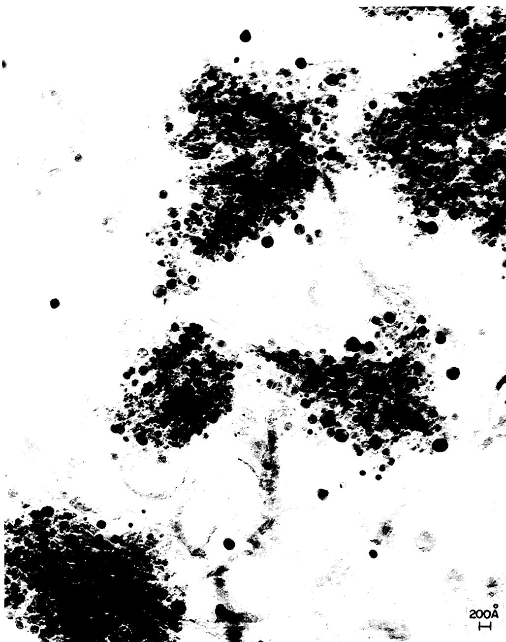
FIG. 4B. Extraction replication showing discrete catalyst particles much larger than clusters of Fig. 4A.
